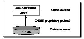
A Java application talks directly to the data source. This requires a JDBC driver that can communicate with the particular data source being accessed. A user's commands are delivered to the database or other data source, and the results of those statements are sent back to the user. The data source may be located on another machine to which the user is connected via a network. This is referred to as a client/server configuration,
